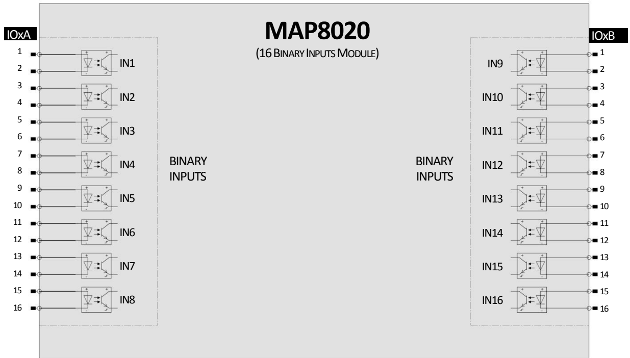
Figure 2.8. MAP8020 expansion module wiring diagram.
