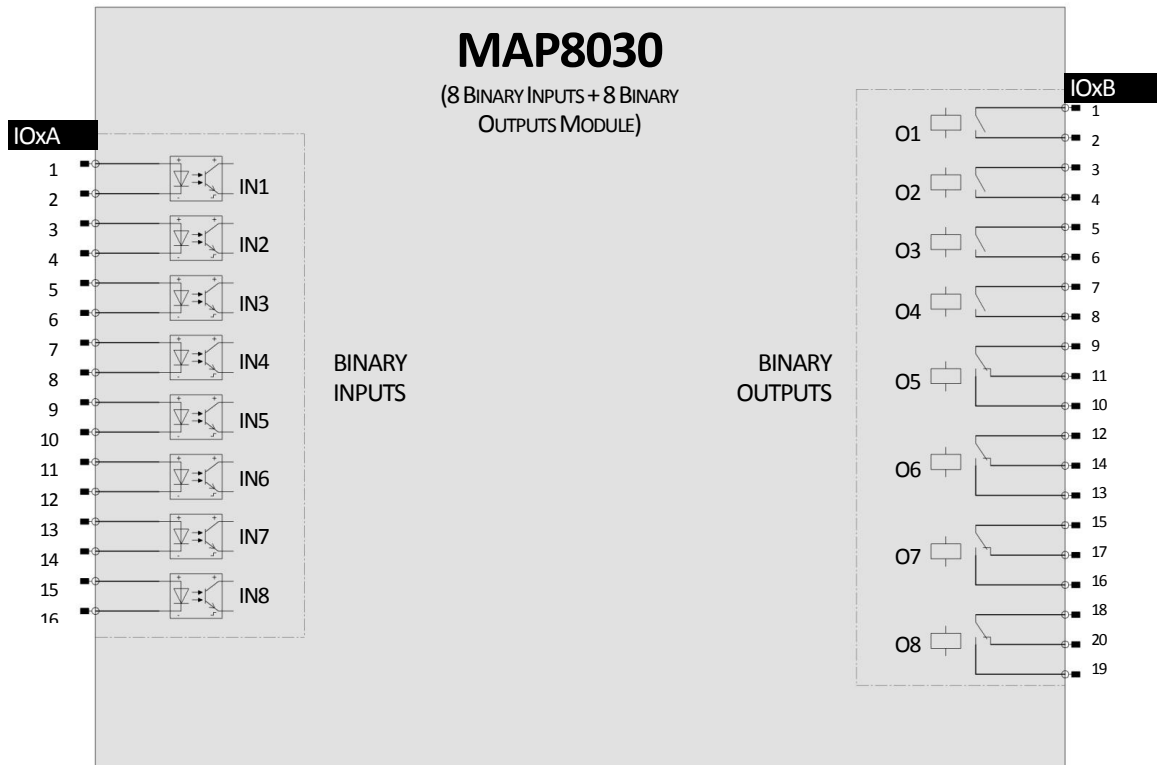
Figure 2.10. MAP8030 expansion module wiring diagram.
