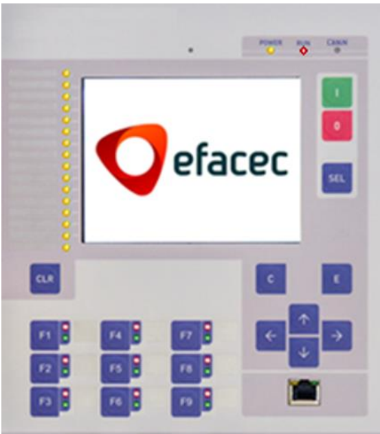
Figure 3.5. Local Human Machine Interface with the red RUN LED marking a complete main hardware failure.
