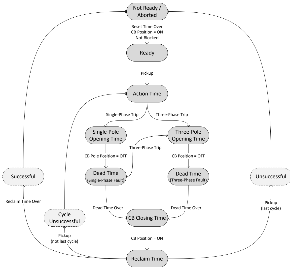
Figure 5.63. Automatic Reclosure state machine.
