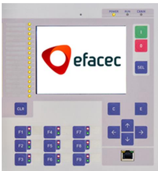
Figure 3.3. Local Human Machine Interface while waiting for startup sequence conclusion.
