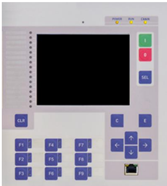
Figure 3.2. Local Human Machine Interface in boot mode.
