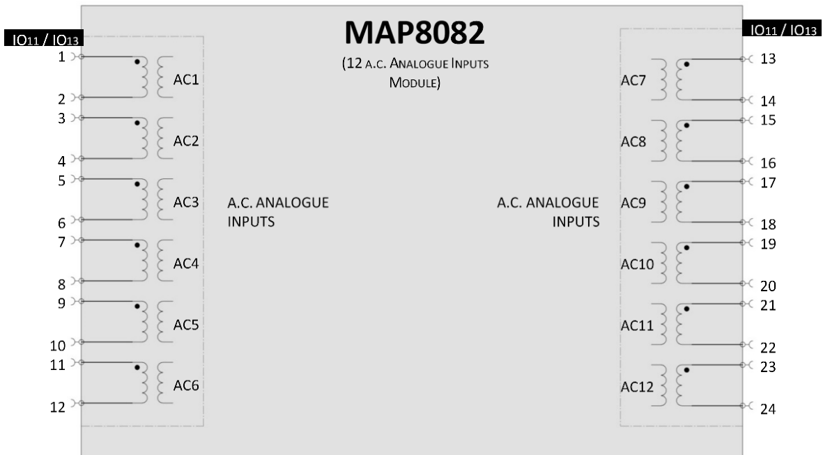
Figure 2.15. MAP8082 expansion module wiring diagram.
