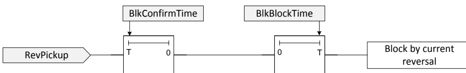
Figure 5.25. Current Reversal logic.
