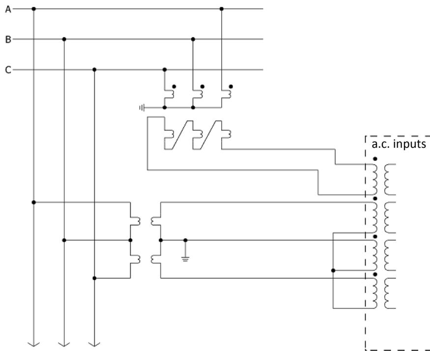
Alternative voltage transformer connection, with three phase-to-earth voltages obtained from two phase-to-phase voltage transformers (Aron circuit). Independent open-delta connected winding is required for residual voltage measurement.
