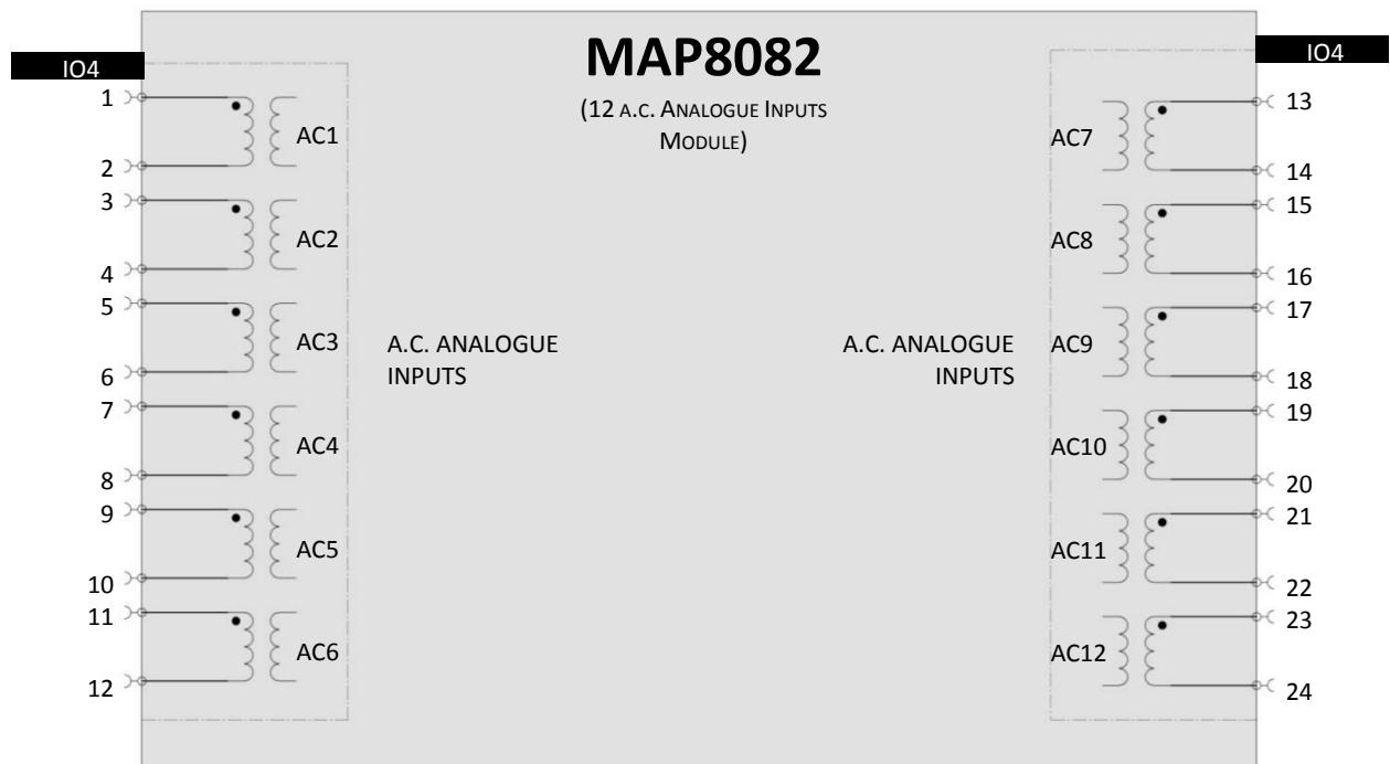
**TYPICAL CONNECTIONS FOR A.C. CURRENT INPUTS**
