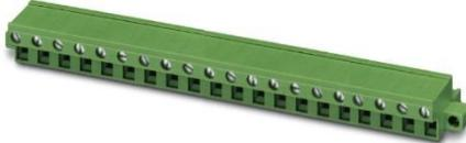
Phoenix Front-MSTB 2.5/20-STF-5.08 (1777976) type connector, 20 contacts. Accepts conductors with section from 0.2 mm<sup>2</sup> to 2.5 mm<sup>2</sup>. The connection is made by screw with the help of a screw driver size 0.6 x 3.5 mm. Tightening torque: 0.5 – 0.6 Nm.
