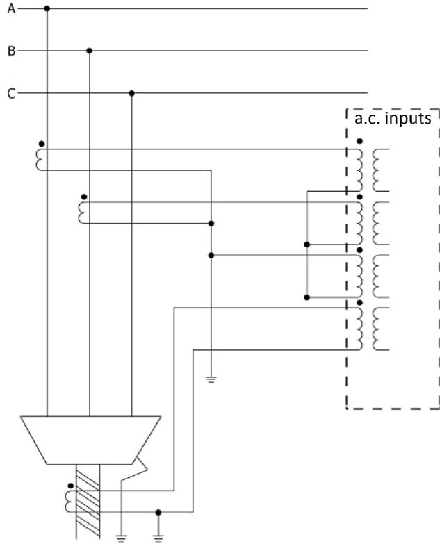
Phase and earth current inputs connection, with current transformers in only two phases. An independent neutral current transformer is required for earth current measurement. Optionally, the third phase current can be obtained from the other two by external circuitry.
