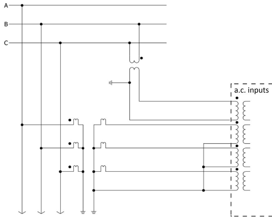
Three phase-to-earth voltage transformer connection and an additional phase-to-phase voltage input for busbar voltage measurement. Fourth voltage connection required for synchronism check applications. Polarization for directional earth-fault protection can be obtained from the internal sum of phase-to-earth voltages.
