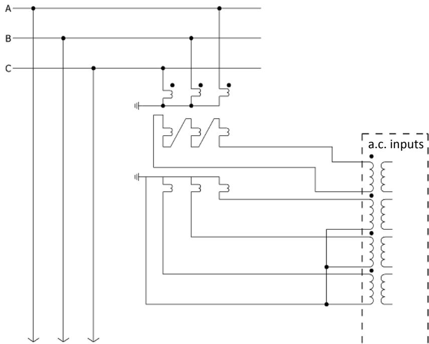
Three phase-to-earth voltage transformer connection, with an independent open-delta connected winding for residual voltage measurement. The fourth voltage input can provide polarization for directional earth-fault protection.
